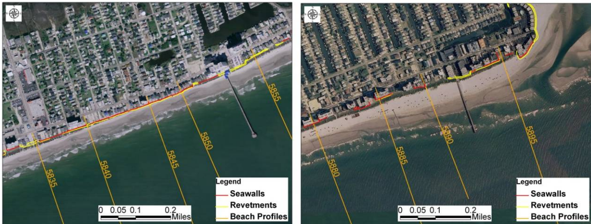
Figures 3 and 4. Region A between Sea Mount Hwy and Cherry Grove Pier (left) and Region B (right) at the northeast extent of North Myrtle Beach adjacent to Hog Inlet. Orange shore perpendicular transects indicate location of SCDHEC-OCRM benchmark profiles. Note: Presence of extensive shoreline armoring in these regions (see Appendix B, OCRM Beach Monuments Map).
