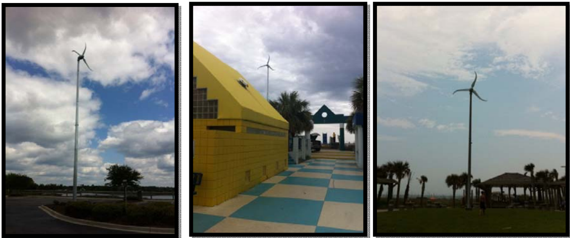
Photos 5-7. Skystream 3.7, 2.4-kilowatt generating wind turbines at Russell Burgess, Jr. Coastal Preserve (left), City Park (middle) and Cherry Grove Oceanfront Park (right).
