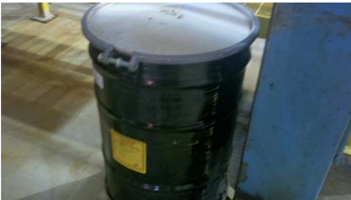
MB1 - Plating Wastewater 90-Day Storage
