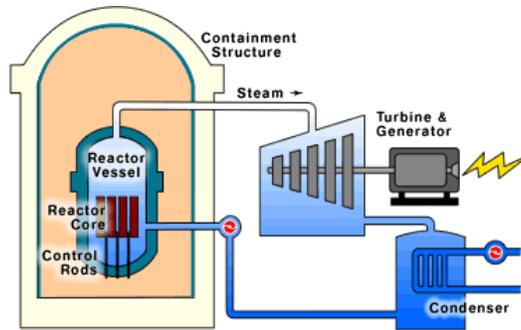
**Pressurized Water Reactors (PWRs)** keep water under pressure so that it heats up but does not boil. Water from the reactor and water in the steam generator never mix.
