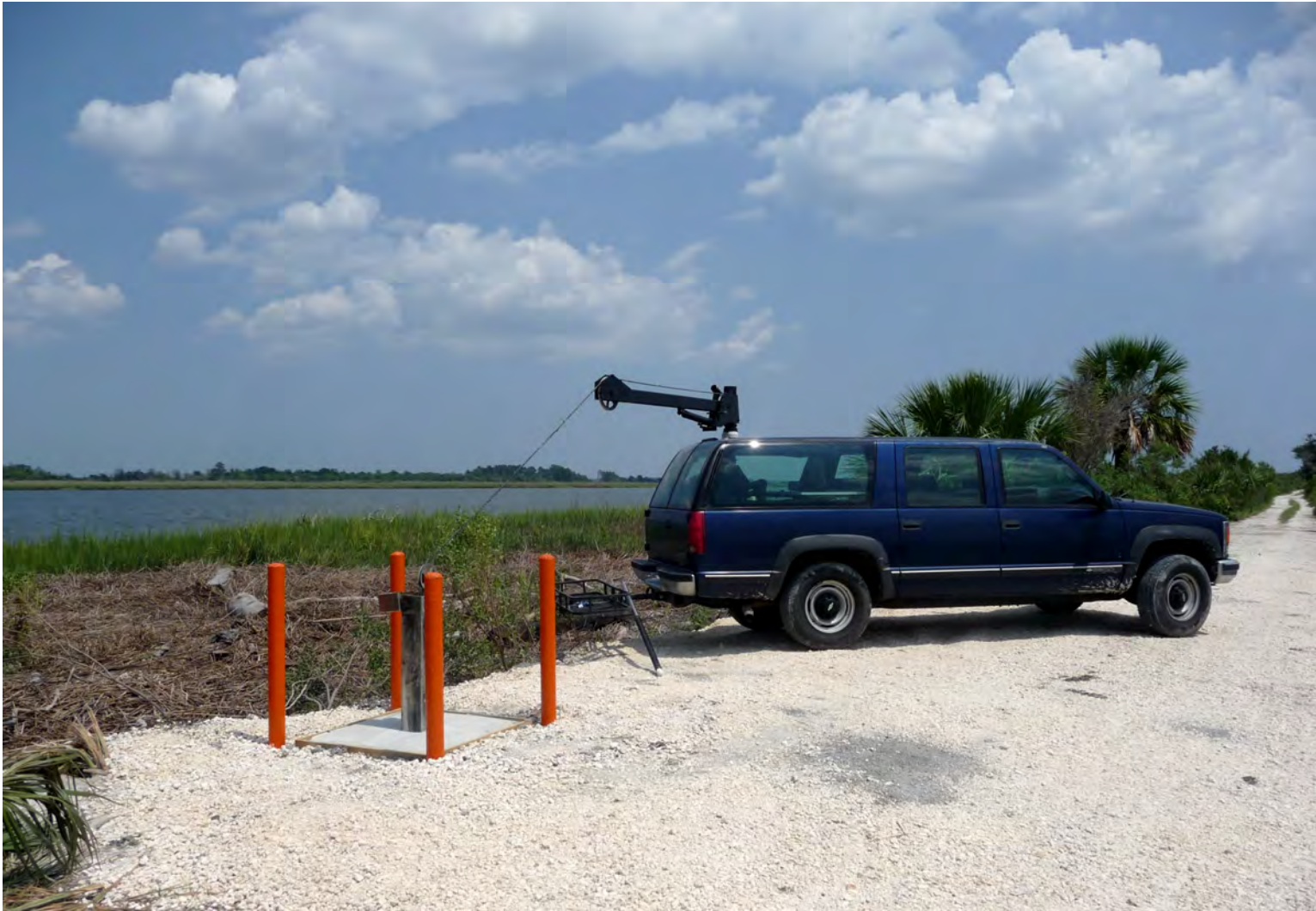
SCDHEC's geophysical logger developed by Mount Sopris Instrument Company preparing to log USACE's monitoring well located on McQueens Island, Chatham County, Ga. Photography by Camille Ransom, III, August 14, 2012.
