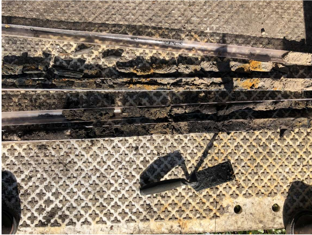
Soil boring samples – January 18, 2022
