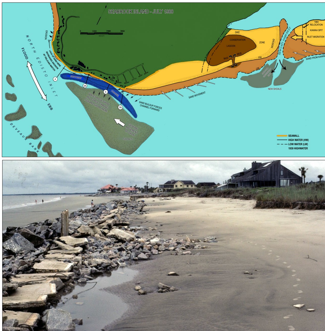
FIGURE 2.7. Conditions along Seabrook Island around 1989 (upper) when the north shoal of North Edisto River Inlet forced the Northern Channel into the seawall and eliminated the wet-sand beach, inhibiting longshore transport to downcoast areas. The lower diagram shows a collapse of the seawall in 1983 in Reach 5.
