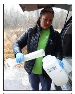
Pouring off a composite sample to be used for monthly alpha, beta, and gamma analysis
