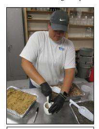
Dried samples are pulverized before being sent to the Columbia lab to be analyzed for radionuclides
