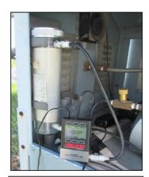
Collecting atmospheric moisture from silica gel through distillation
