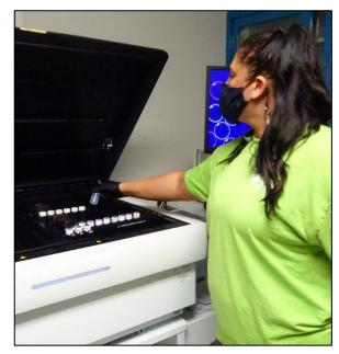
Placing water samples into the Liquid Scintillation Counter to analyze for tritium
