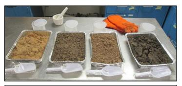
Sediment samples after being placed in drying oven
