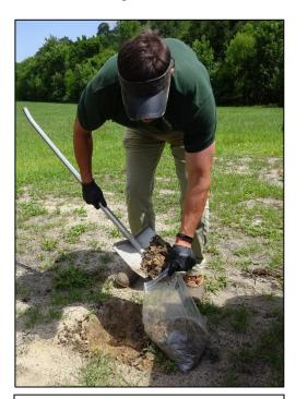
Collecting soil samples which will be analyzed for radiological material and metals
