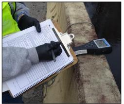
Recording field parameters: DO, pH, temperature, conductivity, and total dissolved solids
