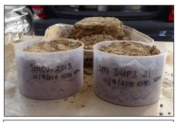
Prepped samples being sent to the lab for radionuclide analysis
