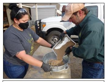
Pieces of rockier sediment are sieved before samples are sent to the Columbia lab for radionuclide analysis
