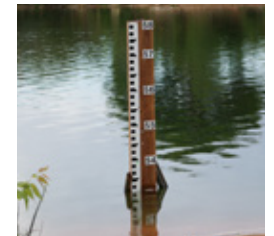
Figure 23. Lake level gauge
