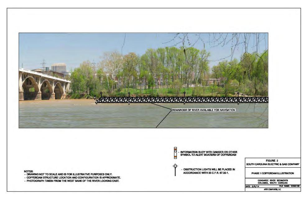
Figure 4. Conceptual drawing showing approximate height and style of proposed coffer dam.
