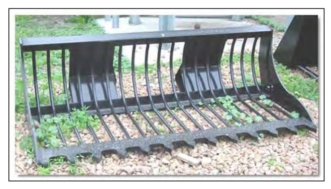
Figure 6. Example of a rock bucket to sort larger artifacts and sort rocks and debris.
