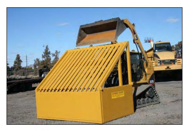
Figure 7. Example of a bar sorter
