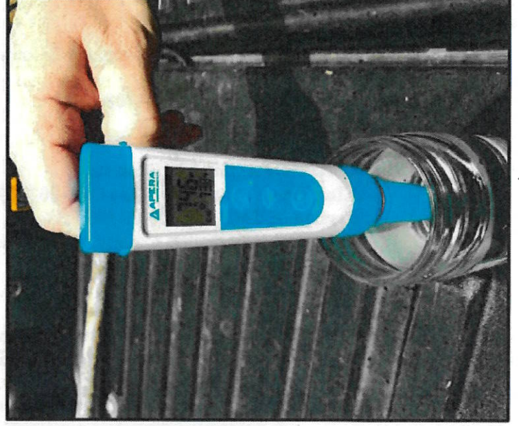
Photo 4: Post-application of Lime pH Sample results from pit (04/20/20).
