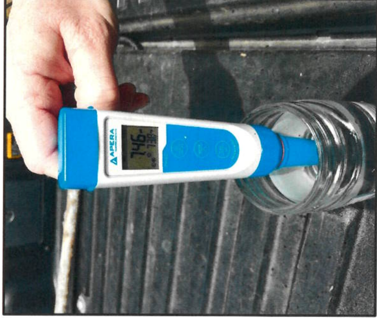
Photo 4: Post-application of Lime pH Sample results from pit (04/20/20).
