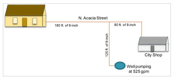
FIGURE 10. Acacia piping arrangement and flow.
