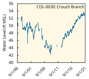
Figure 21. Water level plot from the Crouch Branch Aquifer well in the Lowcountry Area. Water levels are in feet relative to mean sea level MSL).
