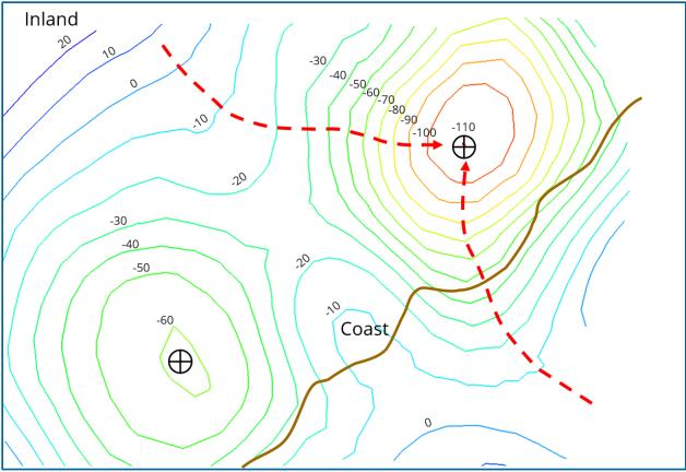
Figure 25. Illustration of a potentiometric map where contour lines show water level elevations from measurements in a confined, coastal aquifer. The numbers in this illustration are elevations in feet relative to mean sea level (the zero contour line). Negative values are feet below mean sea level, and the dashed red arrows indicate the direction of groundwater flow.
