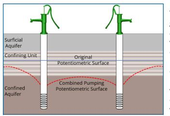
*Figure 24. Illustration of the effect of combined pumping on a potentiometric surface.*
