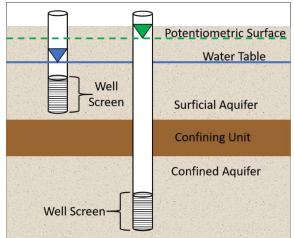
Figure 23. Illustration of a water table and potentiometric surface. Water levels in the wells are indicated by the blue (water table) and green (potentiometric surface) triangles.
