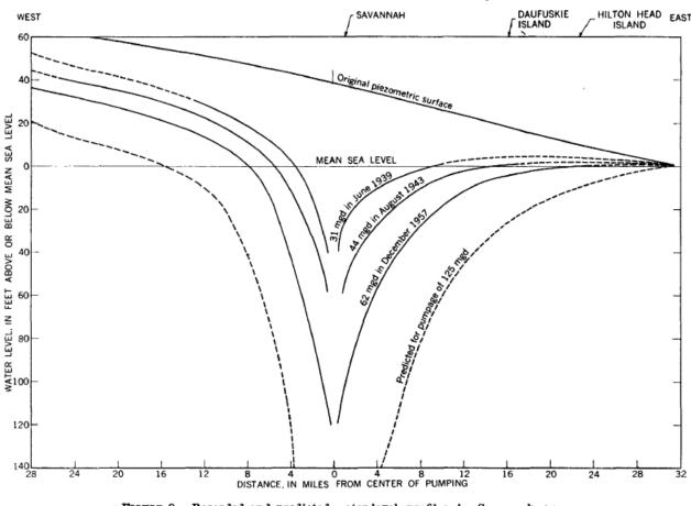
FIGURE 8.---Recorded and predicted water-level profiles in Savannah area.
