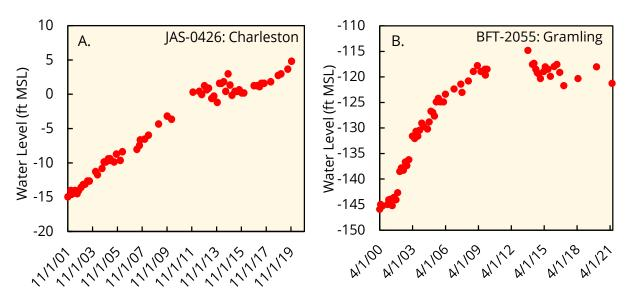
Figure 22. Manual water level measurements in the A) Charleston Aquifer and B) Gramling Aquifer in the Lowcountry Area. Water levels are in feet relative to mean sea level (MSL). <u>http://hydrology.dnr.sc.gov/groundwater-data/</u>; accessed over several days, July 2021.
