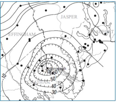
Figure C4. Potentiometric contour lines depicting the state of the Savannah pumping cone in 2010 (Kinnaman & Dixon, 2011). Units are in feet relative to mean sea level.
