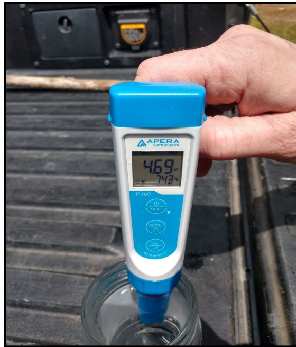
Photo 3: Pre-application of Lime pH Sample results from pit (04/20/20).
