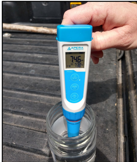
Photo 4: Post-application of Lime pH Sample results from pit (04/20/20).
